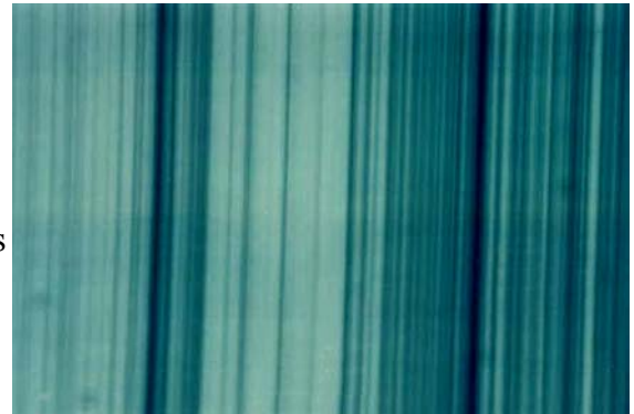
G-Band of CH (methyne)molecule at 4310Å, fully resolved. Color through eyepiece is rich royal blue.
